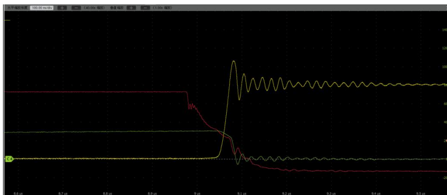
(b) 关断波形, VDD=800V, ID=30A, RG=10Ω, VGS(off)=-3V
